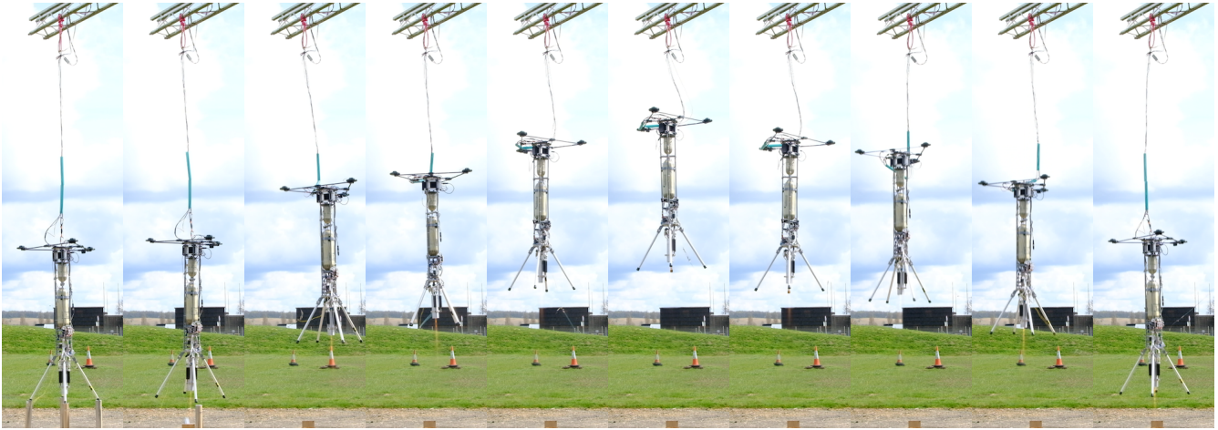
Figure 5: A sequence of stills from a hovering flight under the tether. The stills depict the lift-off and shut-down sequences, the central hovering still are omitted.
