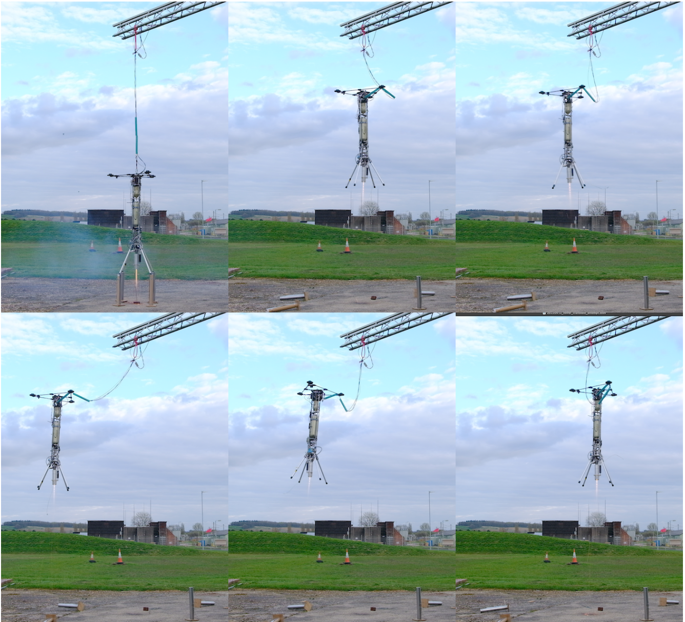
Figure 7: Sequence of stills from a test flight, Top-Left to Bottom-Right: Ignition and self-check, lift off to hovering altitude, begin translation left, hover in new position, begin translation right, hover in original position.
